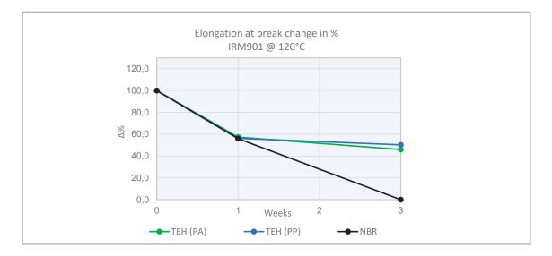
A similar trend can be seen in **figure 6**, which displays the materials' tensile behavior when stored in elevated air temperature for six weeks at 120 °C (248 °F). The products' behavior in an oxidative environment at 120 °C (248 °F) shows significant differences between the performance of TEHs and NBR-based rubber. The durability of NBR-based rubber compounds is already exceeded after three weeks, while the TEHs' tensile strengths remain almost constant over a measuring period of six weeks.
