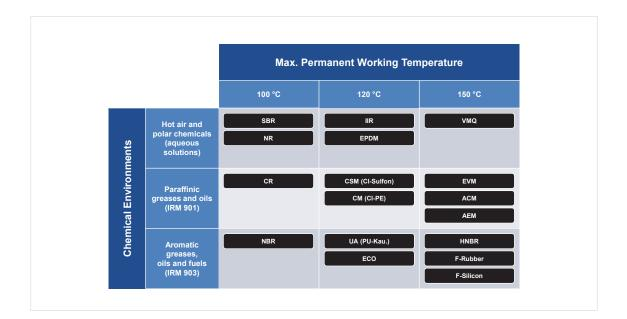
Figure 1: Classification of rubber types based on different elastomers relative to temperature and media resistance
