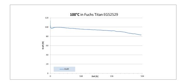
As can be seen from the measurements, the materials are best suited for use in permanent contact with paraffinic oils. Especially at peak temperatures of 120 °C (248 °F), they show better resistance than a comparable NBR-based rubber compound.
